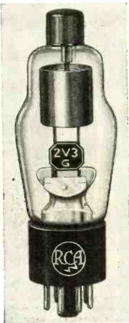
New high-voltage half-wave rectifier for use in television power supply units—type 2V3-G. The peak inverse voltage of this tube is 16,500.
