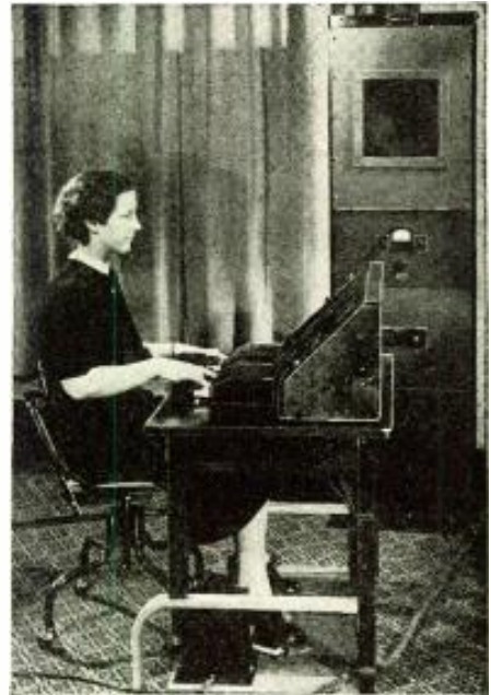
Above: Seated at the keyboard, this young lady can carry on a conversation by pressing keys. A foot pedal changes inflections. The "voice" comes through the loud speaker.
