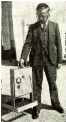
Left — Finished 3-tube ore-locator in use.
